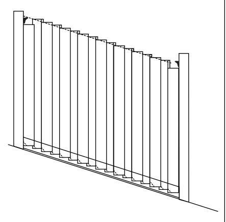
For transitions, you need to cut your pickets at an angle. This is easily done by assembling the pickets and then chalking a line so you can cut them with a circular saw.
